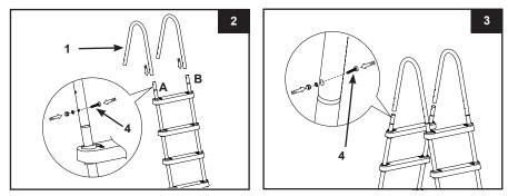
INSTALLATION OF THE REMAINING LADDER SIDE (refer to figure 3):
