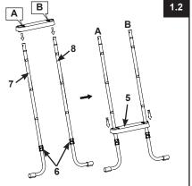
**IMPORTANT:** Ensure the J-shaped legs are pointing outwards before installing the steps.
